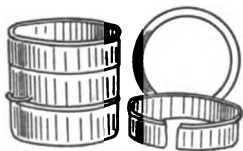
FIG. 78. — A hoop for making "Young America" cheese, a size suitable for the farm.
